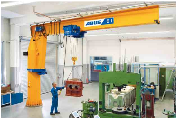
Type E monorail hoist on a type VS pillar jib crane
